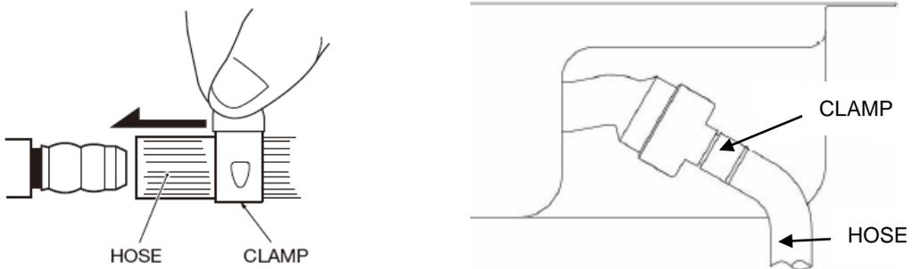
Upon complete of gas installation connections, it is compulsory to check for the gas leakage at the joint with soap test.
