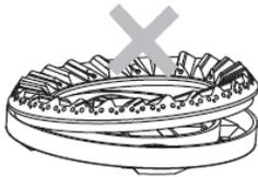
Burner ring is not positioned properly
